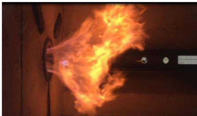
Figure 12 – Torch of flame obtained by burning biogas in a laboratory installation
