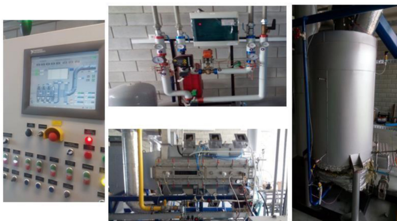
Figure 13 – Two-level structure of the automated system for diagnosing and controlling the process of biogas combustion in laboratory conditions of the Lublin University of Technology (Lublin, Poland)
